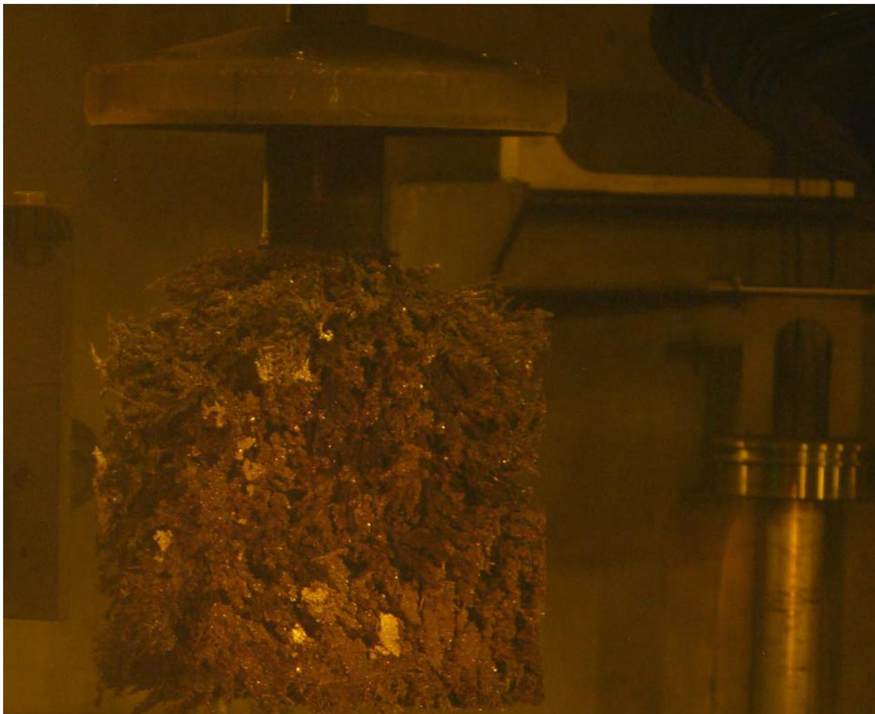
*An impure uranium waste product is deposited on a cathode in a pyroprocessing cell (Source: Idaho National Lab)*
