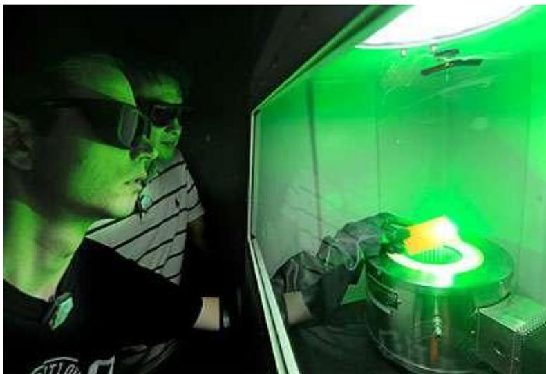
*Laser-Induced Breakdown Spectroscopy uses a high-power laser within the Center for Advanced Energy Studies at INL. The technique can discern the contents of used nuclear fuel and potentially boost the global security of nuclear recycling. Credit: Post Register*
